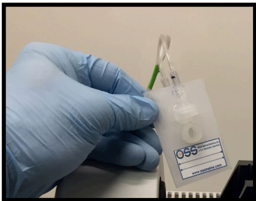
Figure 1: OSS Extractor in an FTIR card holder and environmental control system
