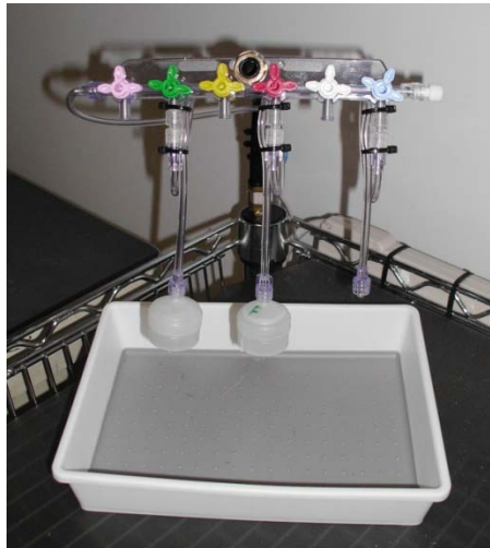
Figure 5: OSS Drying Manifold
