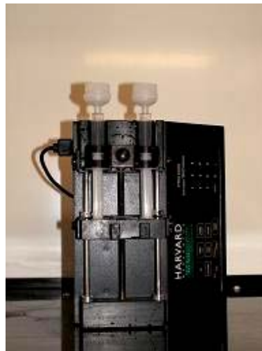
Figure 4: Extractors attached to sample syringes.
