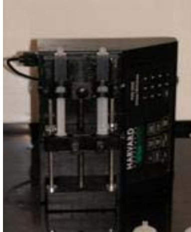
Figure 3: Syringe pump loaded with two sample syringes
