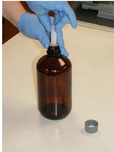
Figure 2: Fill syringe with at least 12 mL of sample
