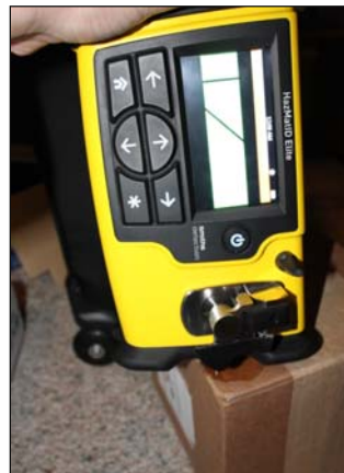
Figure 6. Interrogation of liquid on cardboard box using the integrated Touch-To-Sample (TTS) sensor.
