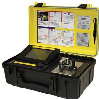
Figure 1. The HazMatID 360 FTIR chemical identification system.
