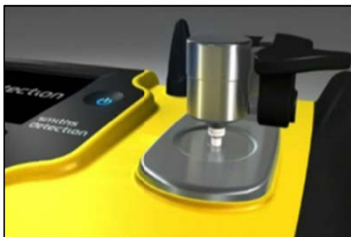
Figure 4. HazMatID Elite integrated press with liquid well
